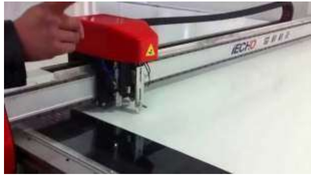
Cutting for PVC membrane structure with large format and high speed
